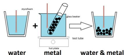
5. Let the water boil for five minutes ensuring that the temperature of the metal inside the test tube is in equilibrium with the boiling water.
